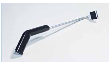
Pedal force meter, model: C_PFM 1000
