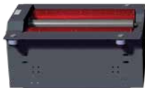
Digital roller brake tester C_MBT S 15.0 R100 MU with two-part roller set, up to 15.0 t axle load and a roller length of 1000 mm, motor positioned under the roller set.
