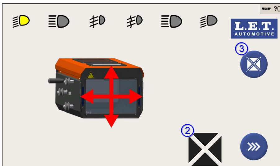
Figure 46: Position Check Arrows on control panel screen
