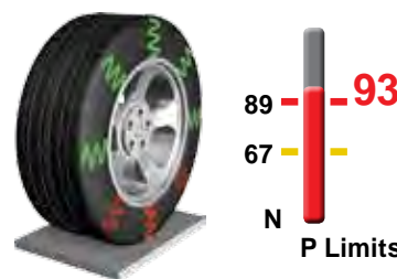
Road Force panel displays assembly value and limits
