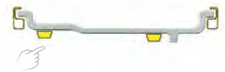
Rim cutaway displays selected weight mode
